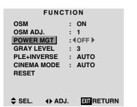
3. To turn the power management function on ... Use the ◀ and ▶ buttons to select "ON". The mode switches as follows each time the ◀ or ▶ button is pressed:
